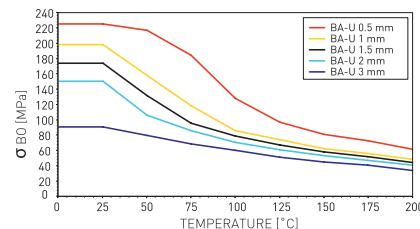
$\sigma_{B0}$  diagrams represent  $\sigma_{B0}$  values for different gasket material thicknesses. These values indicate the maximum in-service compressive pressures which can be applied on the gasket area involved without destroying or damaging the gasket material.
