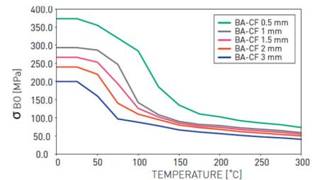
σ<sub>BO</sub> diagrams represent σ<sub>BO</sub> values for different gasket material thicknesses. These values indicate the maximum in-service compressive pressures which can be applied on the gasket area involved without destructing or damaging the gasket material.
